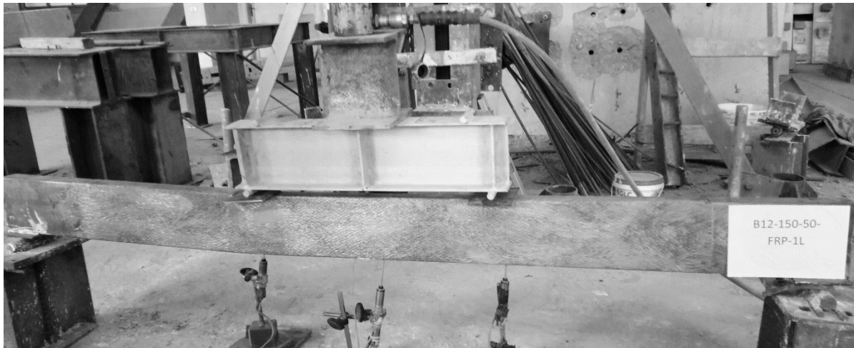
A.) OVERALL PICTURE OF SPECIMEN B12-1L DURING FAILURE
