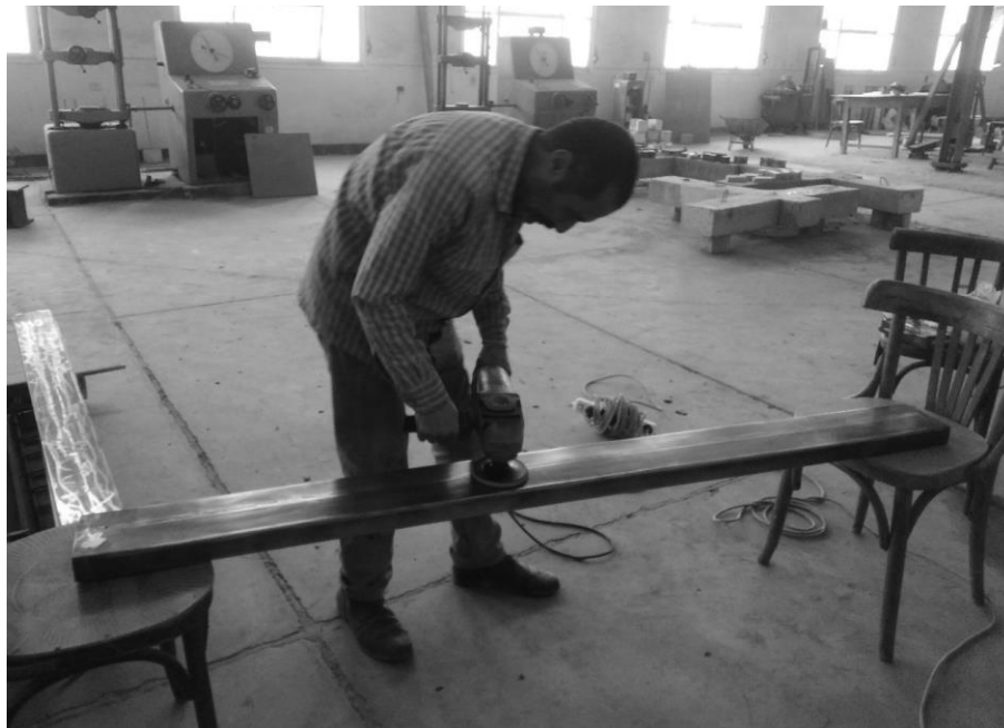
FIGURE 3. PROCESS OF PREPARING STEEL SURFACE USING SAND PAPER.
